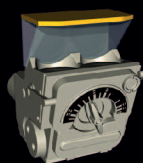
Q32247 Gyro gunsight Mk.II for late Tempest and other fighters
