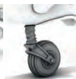
Q72391 Bf 109E Tailwheel with Strengthened Leg
